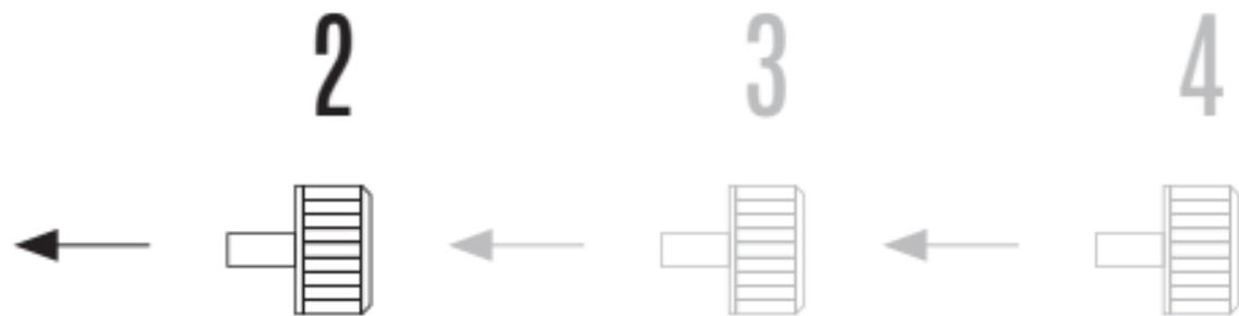
*The crown must be screwed down in position 1 for optimal water-resistance.*
